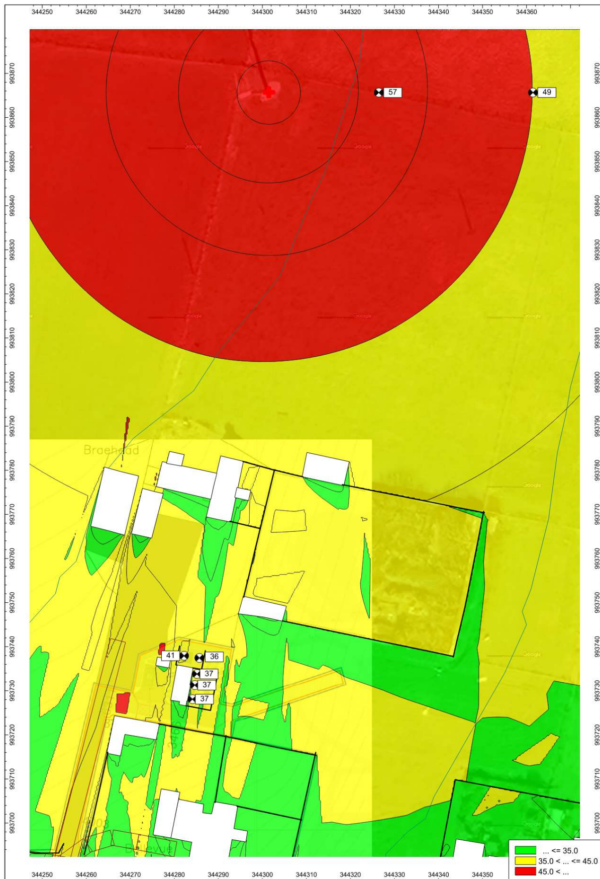
Figure A.3 – Turbine noise emissions L_{A90,10\text{mins}} – grid height 1.5m – wind speed 10 m/s
