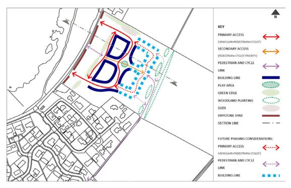
Proposed Layout Plan showing development phases outlining access and linkages
