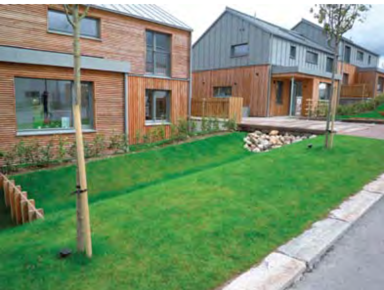
Contemporary use of materials and swales used as part of a SUDS system
