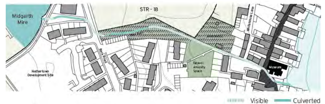
Figure 5: Mayburn Culvert Plan
