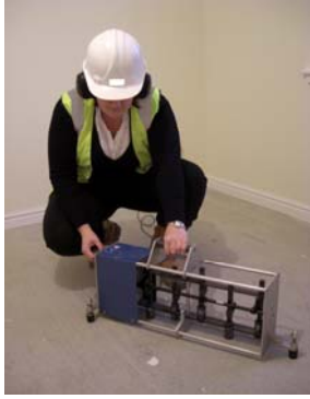
Fig. 4 Impact sound test being carried out
