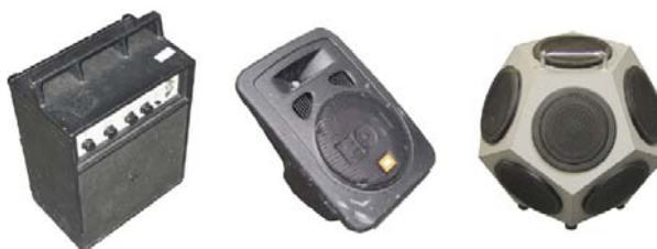
Fig. 3 Typical loudspeakers used during airborne sound insulation tests
