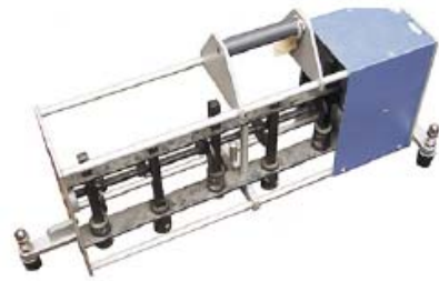
Fig. 5 Typical tapping machines for impact sound insulation tests
