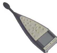
Fig. 2 Typical sound level meter for measuring sound insulation
