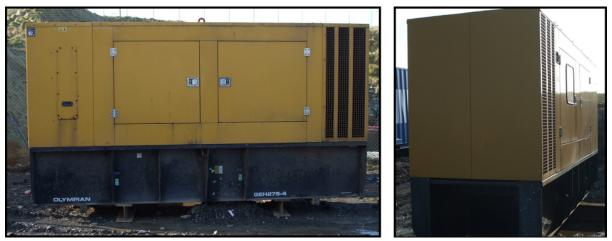
Olympian GEH275-4 generator, 200kW, 400 v (3 phase), 275 KVA, manufactured 2012 with approximately 9068 working hours.
